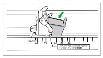
**5.** Lock the ink cartridge adjustment lever (1).
